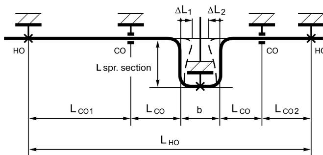
The compensation of thermal extensions is solved constructively, using angles of rotation, sliding and fixed supports, as well as ready-made expansion joints. In fixed supports, the pipe is rigidly fastened with a collar with rubber gasket, and in sliding supports, retainers allow the pipe to move in the axial direction.
