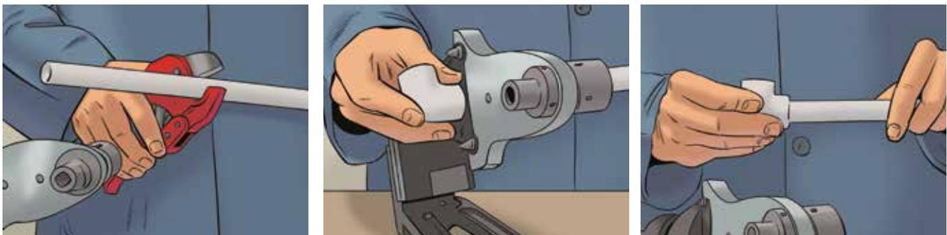
1. The welding adaptors of the appropriate diameter are installed on the welding machine after making sure that the working surfaces of the welding adaptors are degreased with acetone or an aqueous solution of alcohol. In cases of sticking of polymer residues from the previous welding, it is necessary to clean the working surfaces.
