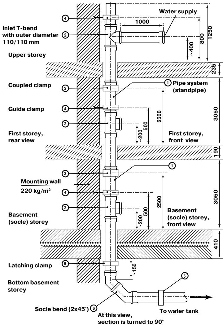
To assess the noise, which the system will generate under the real operating conditions, tests under EN 14366 are conducted, in which a portion of multi-apartment building is simulated.
